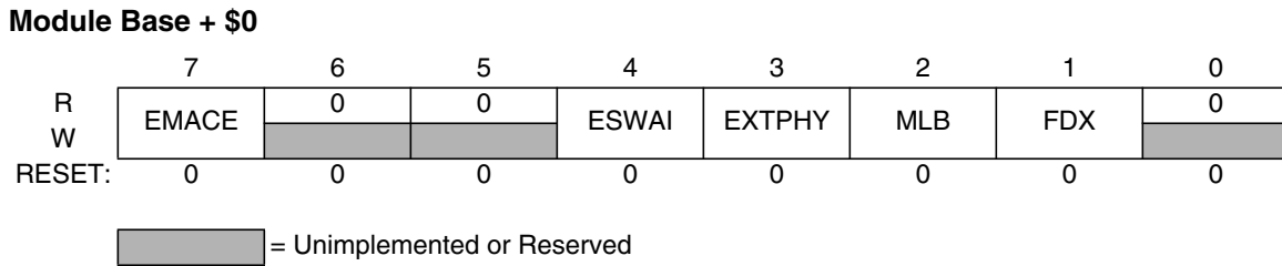
Figure 11-2. Network Control (NETCTL)
